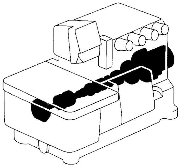
B. 駆動軸関係/Crank shaft mechanism/Kurbelwelle/
