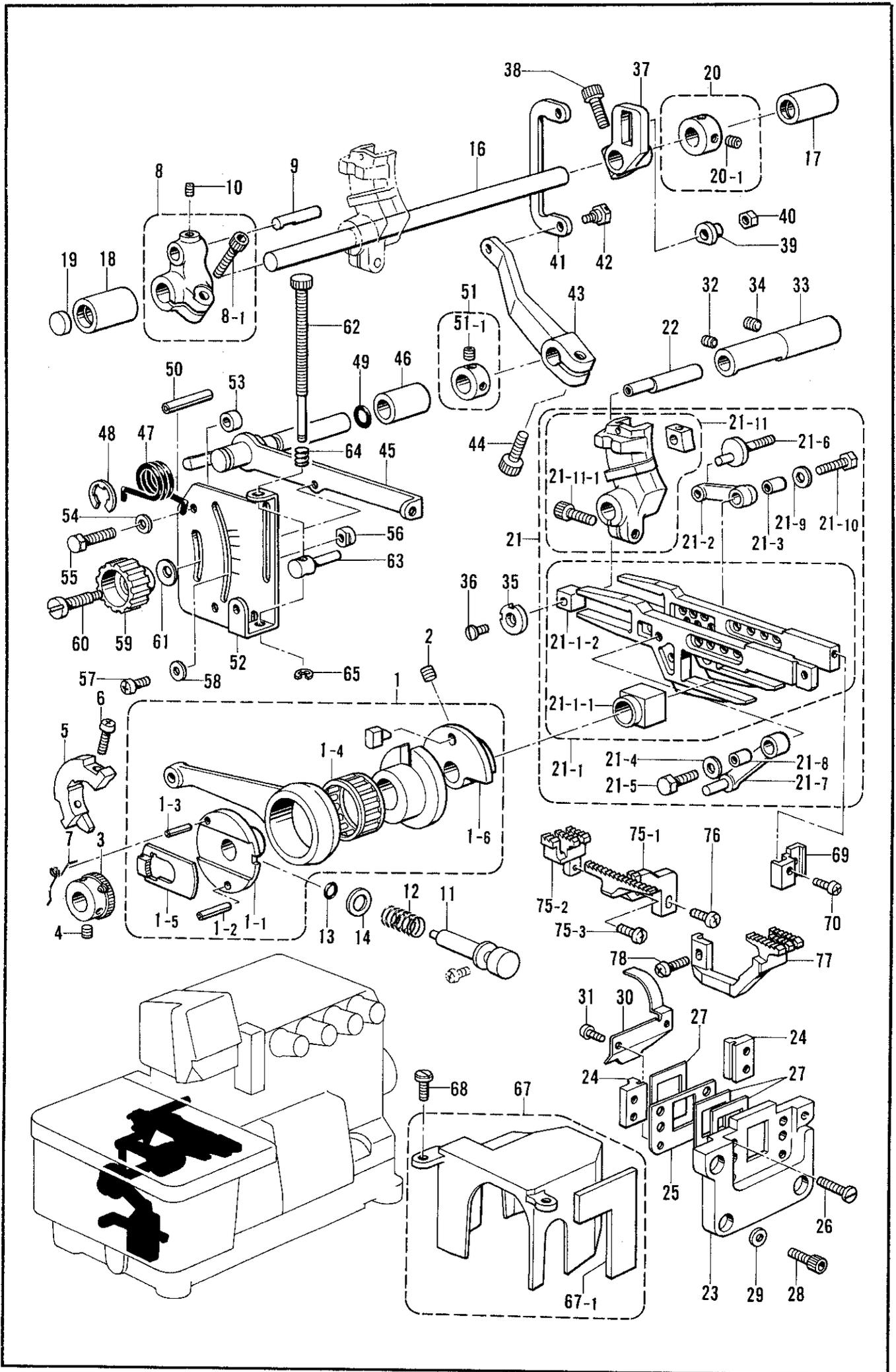
E. 送り関係/Feed mechanism/Transportvorrichtung/
