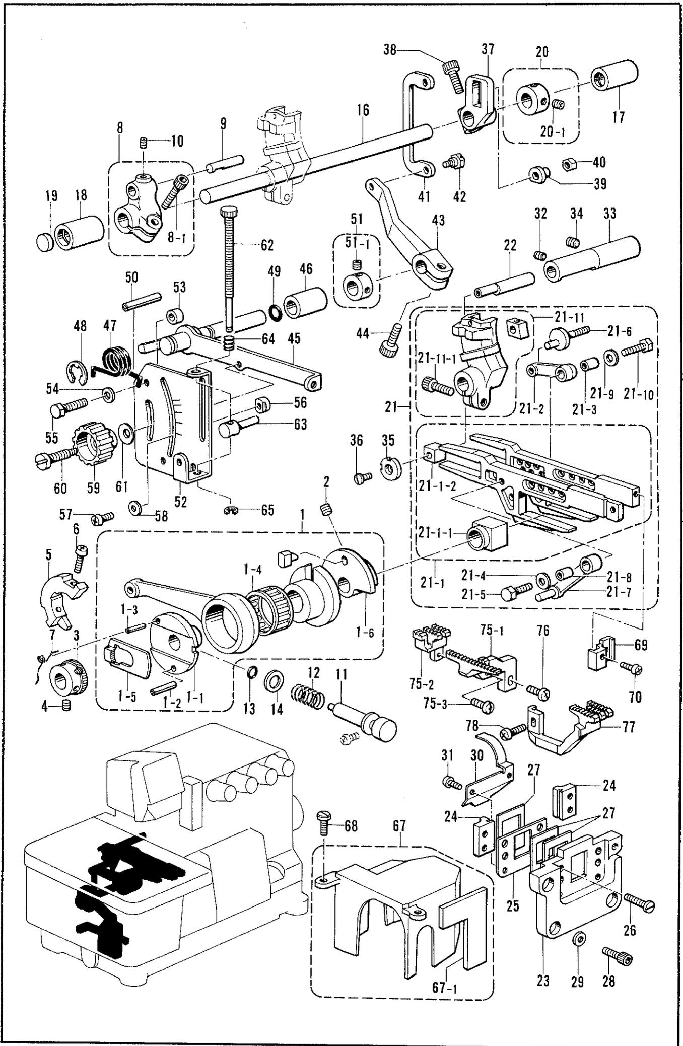
E. 送り関係/Feed mechanism/Transportvorrichtung/
