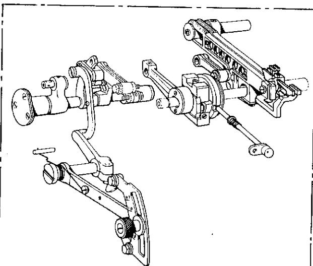
F. 送り関係/Feed mechanism/Transportvorrichtung/
