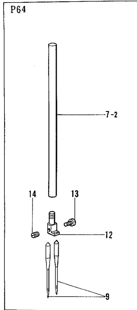
C. 針棒関係/Needle bar mechanism/Nadelstangenvorrichtung/
