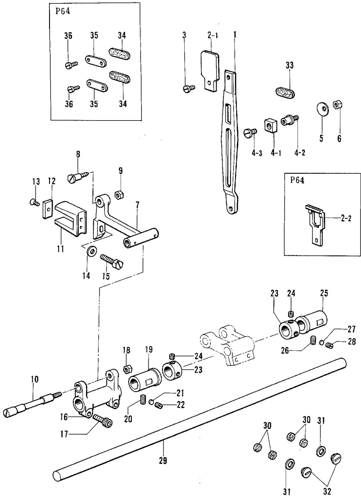
G. 送り軸関係/Feed shaft mechanism/Transport welle/
