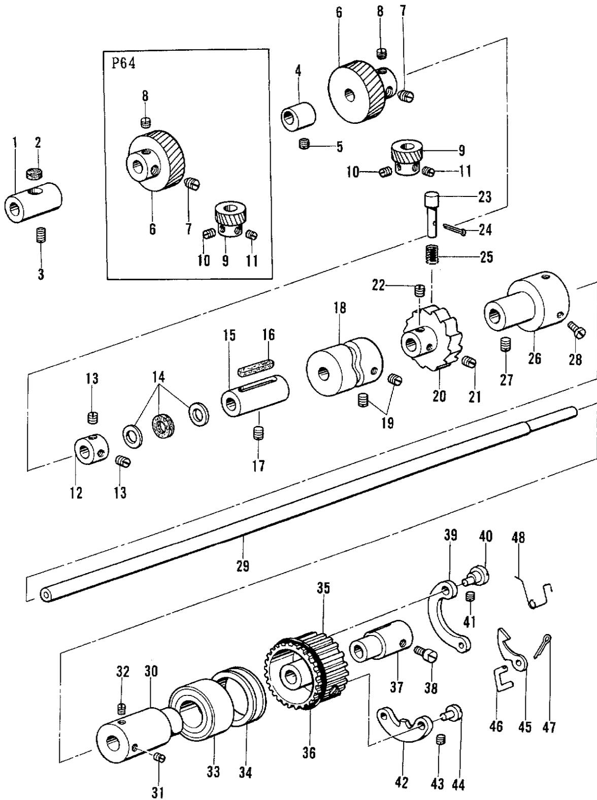
H. 下軸関係/ Lower shaft mechanism/ Untere Welle/
