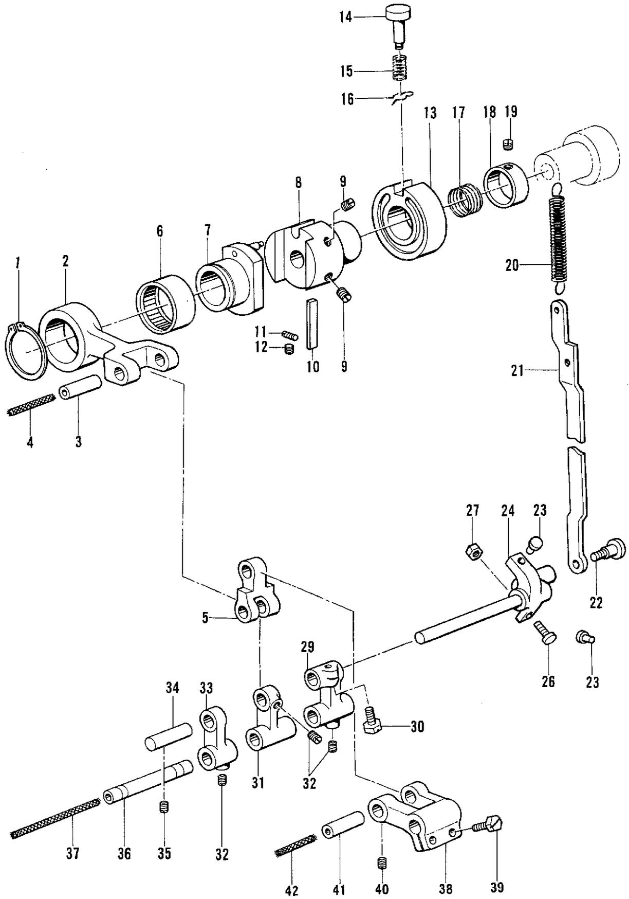
F. 送り関係/Feed mechanism/Transportvorrichtung/
