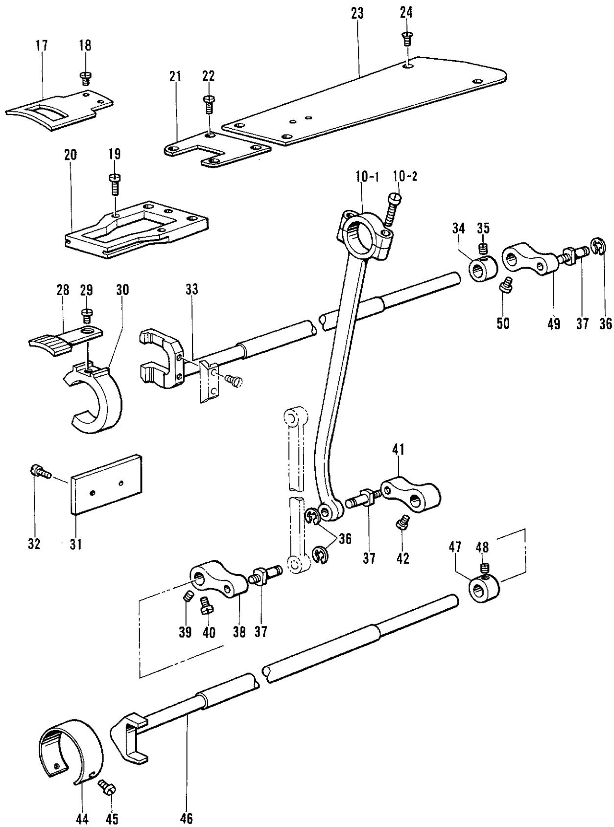
H2. 送り関係 /Feed mechanism/Transportvorrichtung/
