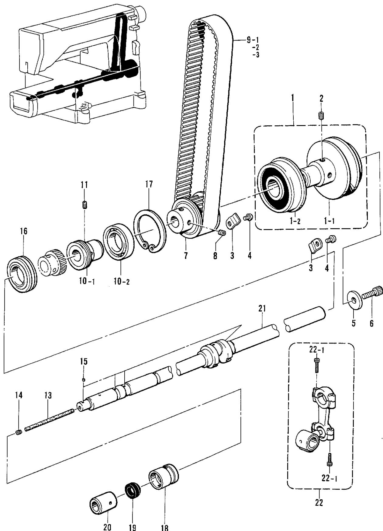
F. 下軸関係/Lower shaft mechanism/Untere Welle/
