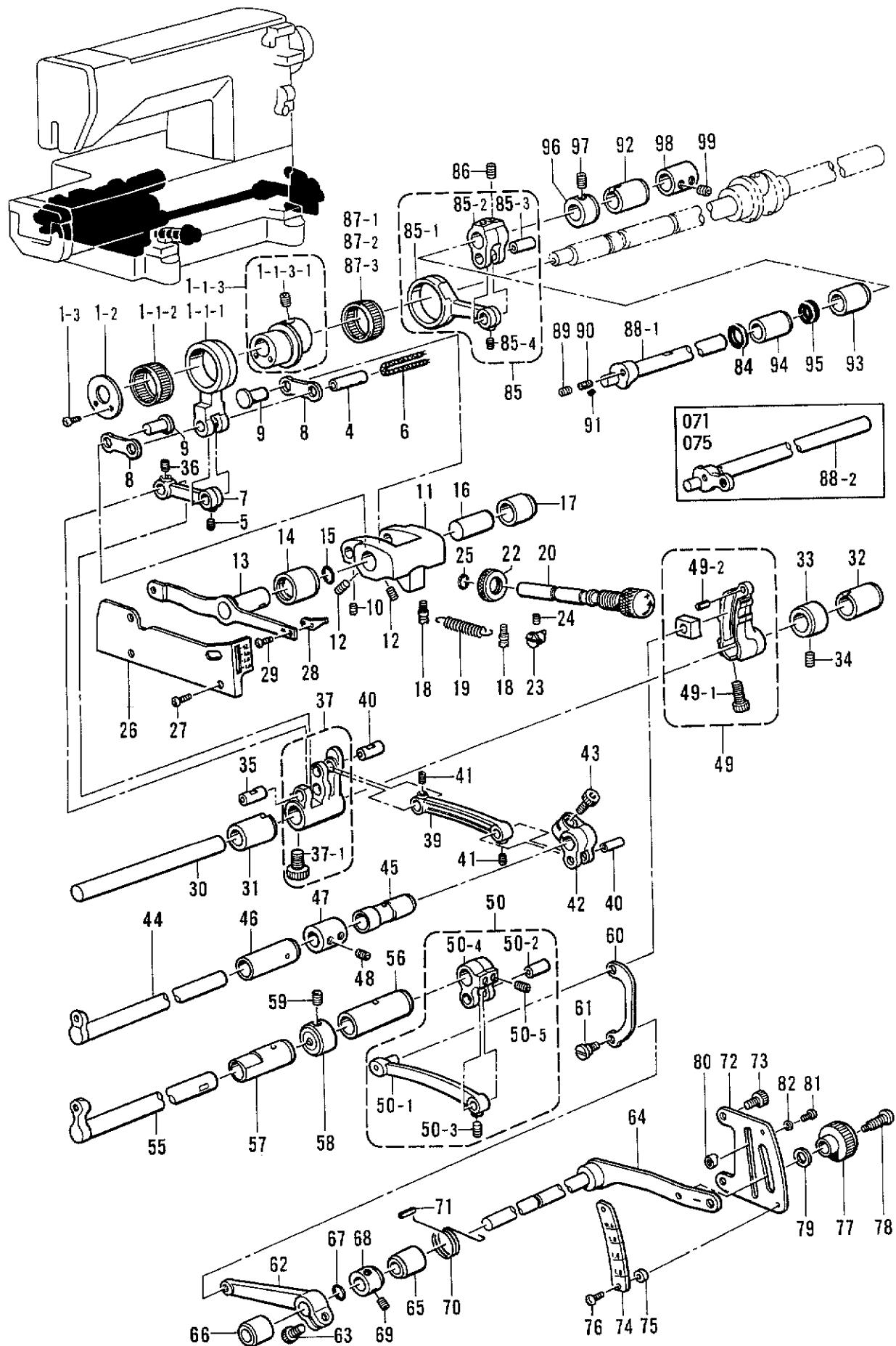
E1. 送り関係 /Feed mechanism/Transportvorrichtung/
