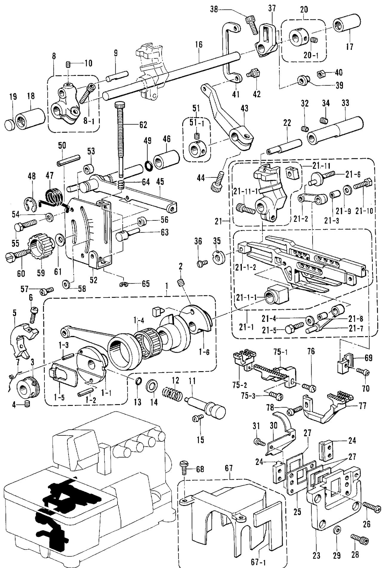
**E. 送り関係 / Feed mechanism / Transportvorrichtung /
