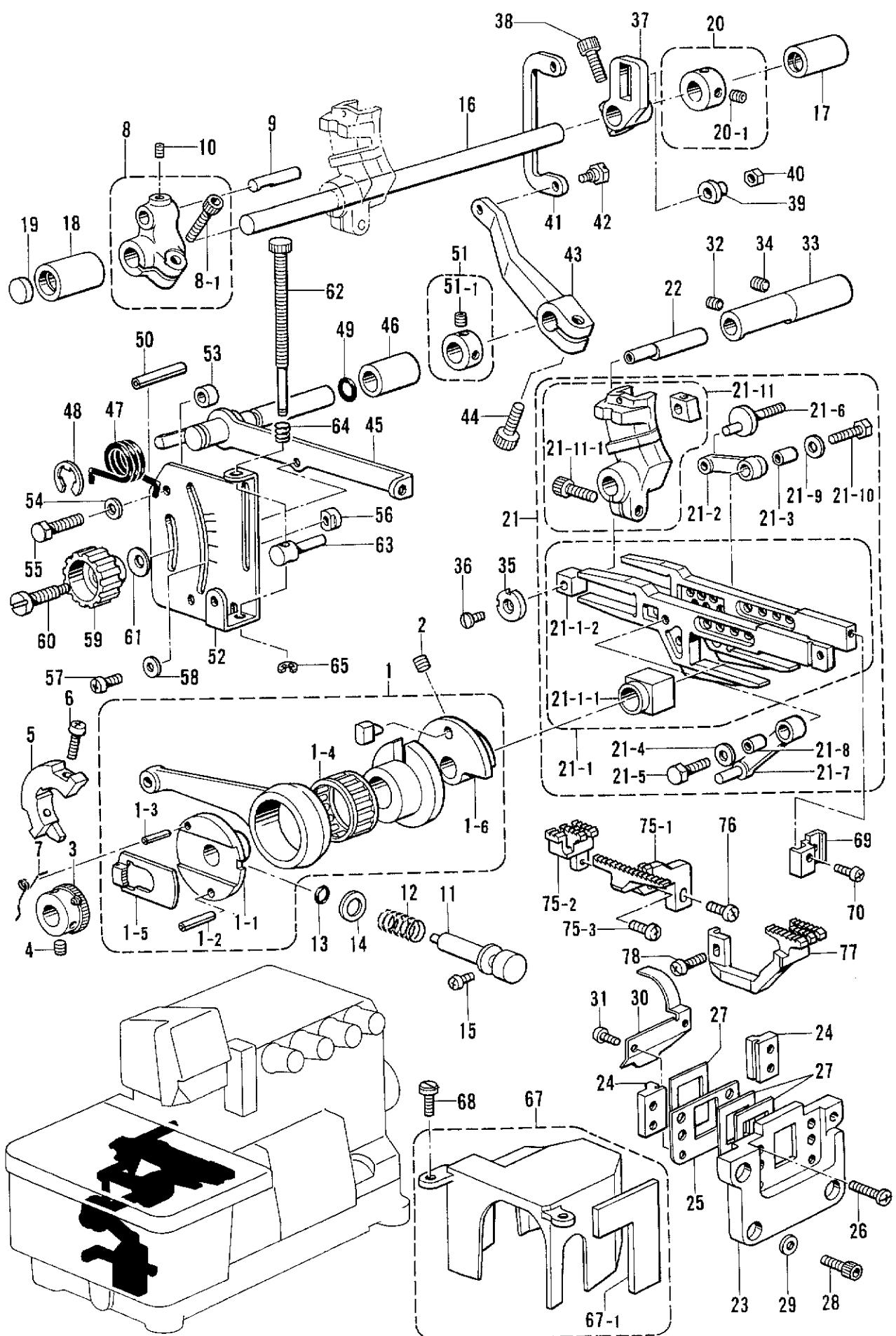
E. 送り関係/Feed mechanism/Transportvorrichtung/
