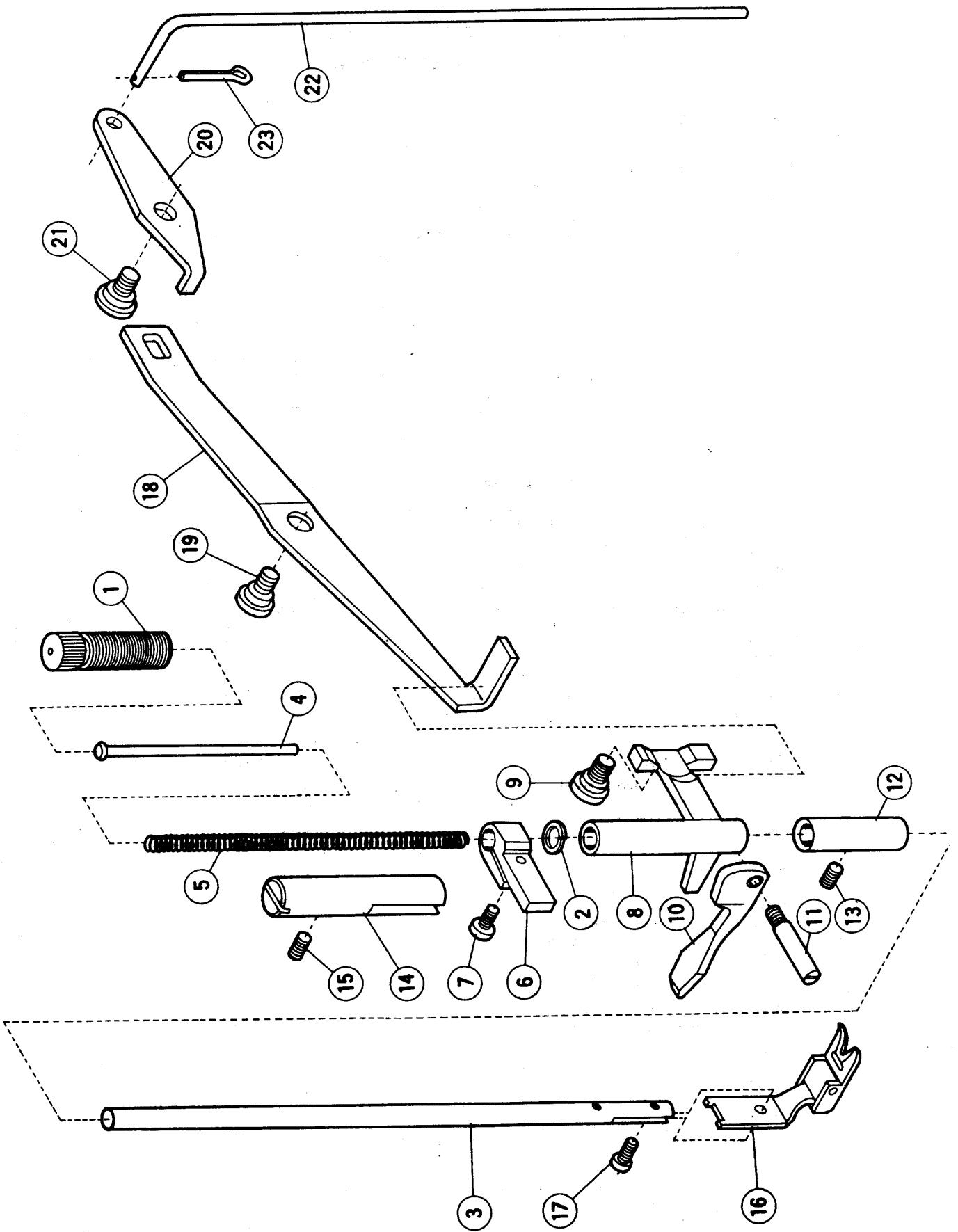
PRESSER FOOT AND LIFT MECHANISM
