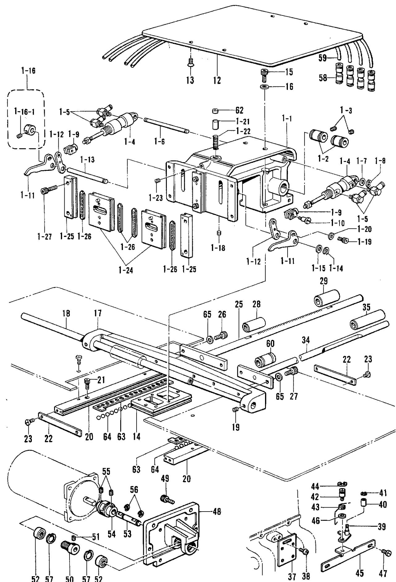
D1. 送り関係 / Feed mechanism (1) / Transportvorrichtung (1) /
