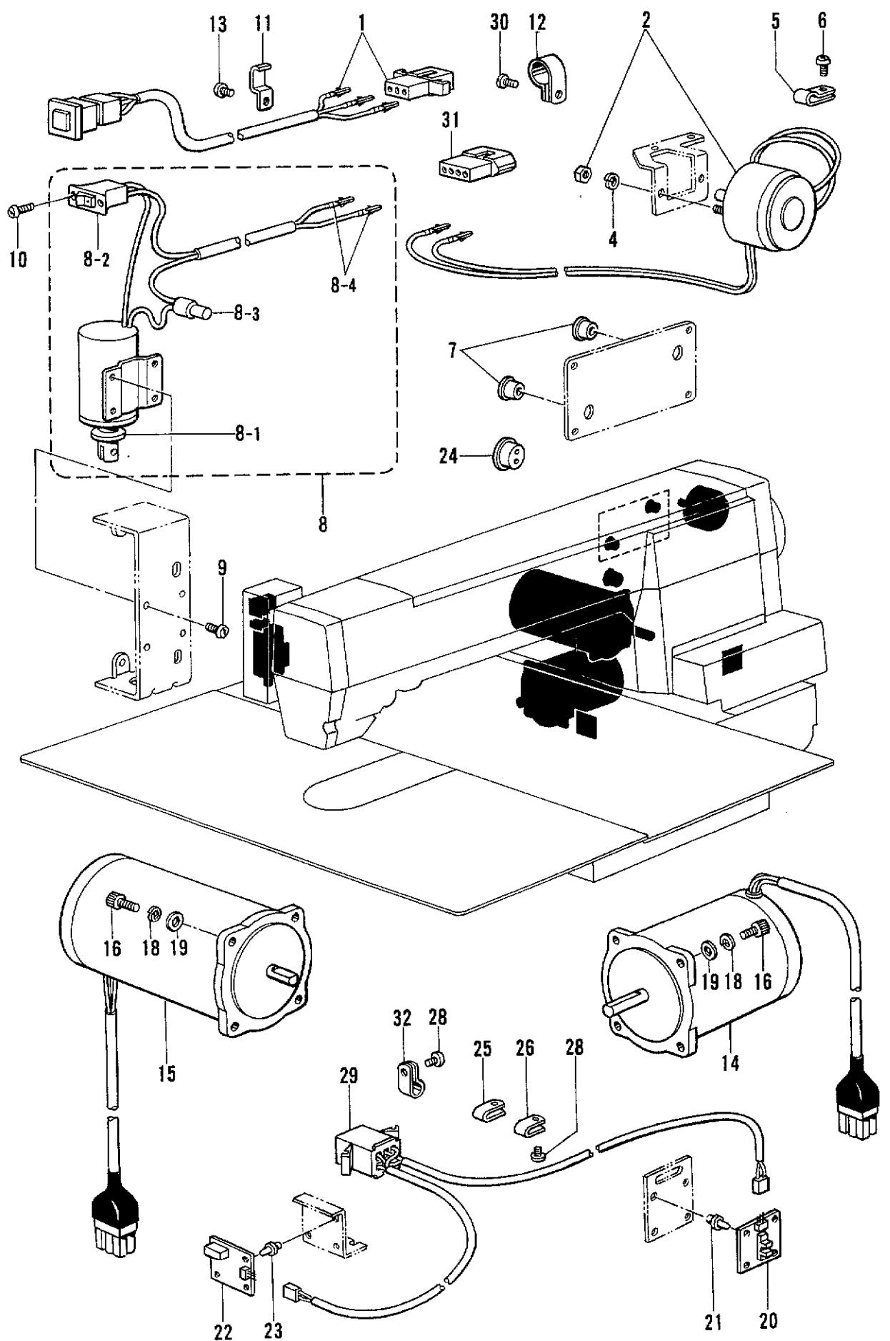
Q. 電装品関係/Power supply equipment mechanism/Stromversorgung/
